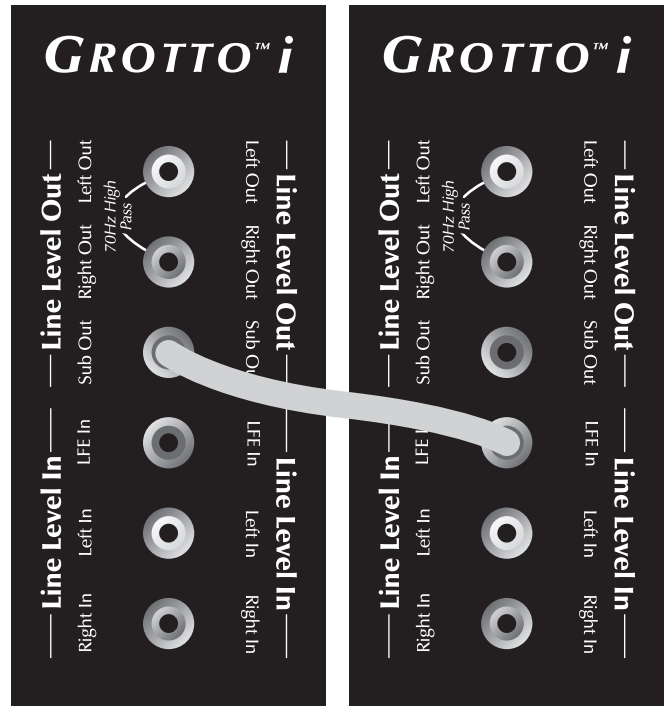
Figure 10. Using multiple Grotto i. LFE option. Primary sub on right. Additional sub on left.
